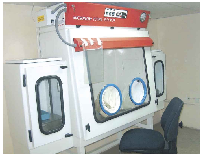
Negative pressure isolator
